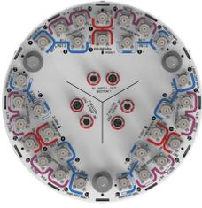
30-ports tri-sector antenna, 6x 698-896, 12x 1695-2200 and 12x 3300-4000 MHz, 65° HPBW, 9x RETs, 6x SBTs.
