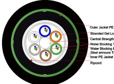
Stranded Gel Loose Tube Central Strength Member Water Blocking Tape/Yams Water Blocking E-Glass Yarn Steel armoure Tape Inner PE Jacket
