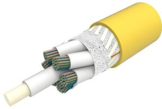
Fiber indoor cable, All-Dielectric, LSZH Riser-Rated, Gel-Free, Loose Tube Rollable Ribbon, 1728 fiber, Singlemode G.657.A2, Feet jacket marking, Yellow jacket color
