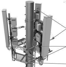
Mounting to Round Member for cable support Material ID: PGP-series cable support brackets, SA-3C, SA-4C, SA-1C, UHA-3C, FBR-COIL-S
