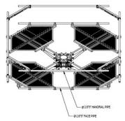
PIM Optimized Adjustable 4-Sector Monopole Platform with 13ft Face - 2-7/8in OD Face Pipes & Top Rail - No Antenna Pipes Included
