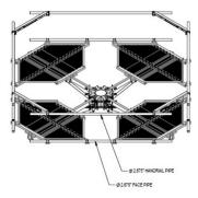
PIM Optimized Adjustable 4-Sector Monopole Platform with 15ft Face - 2-7/8in OD Face Pipes & Top Rail - No Antenna Pipes Included
