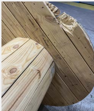
Do not return a cable reel with a damaged flange.
