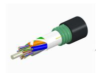
Fiber OSP cable, LazrSPEED® Single Jacket/Single Armor, 144 fiber, Gel-Free, Stranded Loose Tube, Multimode OM4, Feet jacket marking, Black jacket color
