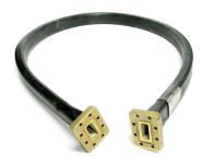
FlexTwist® Flexible Twist for WR62, 12.4–18.0 GHz, with interface types PBR140 and PBR140, 300 mm
