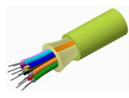
Fiber indoor cable, LazrSPEED® Low Smoke Zero Halogen Riser Distribution, 6 fiber single-unit, Multimode OM5, Feet jacket marking, Lime green jacket color, Dca flame rating
