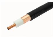
RCT6, RADIAX® Coaxial Radiating Cable with Bump, 50–900 MHz, tuned foil, 1-1/4 in, black non-halogenated, fire retardant polyolefin jacket
