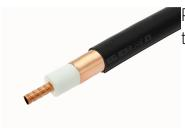
RCT6, RADIAX® Coaxial Radiating Cable with Bump, 70–960 MHz, tuned foil, 1-1/4 in, black non-halogenated, fire retardant polyolefin jacket
