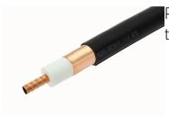
RCT6, RADIAX® Coaxial Radiating Cable with Bump, 1700-2500 MHz, tuned foil, 1-1/4 in, black non-halogenated, fire retardant polyolefin jacket
