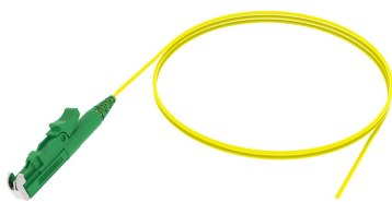
Fiber Optic Pigtail, Simplex, Singlemode, LSH/APC to Stub, yellow, 6 m
