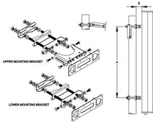
Adjustable Tilt Pipe Mounting Kit for 2.0"-4.5" (60-115mm) OD round members for panel antennas. Includes 2 clamp sets.
