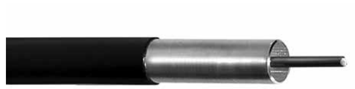
conductor clean of dielectric and bonding compounds after coring
