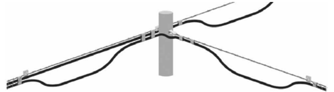
LINE POLE DEAD-END
