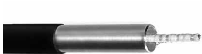
residual dielectric and bonding compound on conductor after coring
