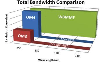
Figure 6 - Conceptual bandwidth comparison
