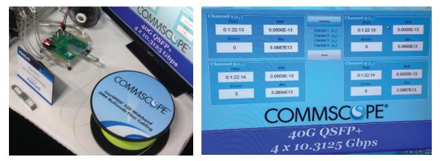
Figure 10 - 40G-SWDM4 over 500 m of LazrSPEED 550 WideBand MMF at BICSI
