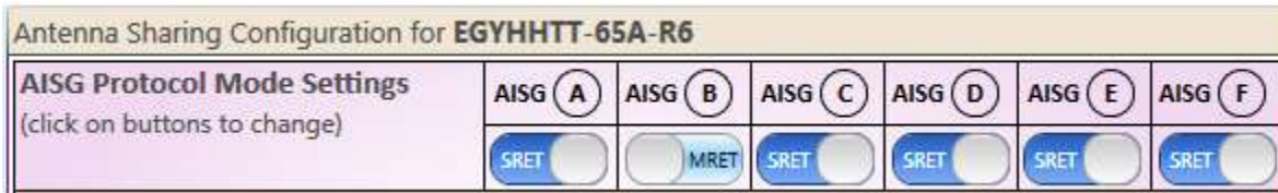
Figure 16 Changing BTS/RRH Control port protocol modes for given antenna model.
