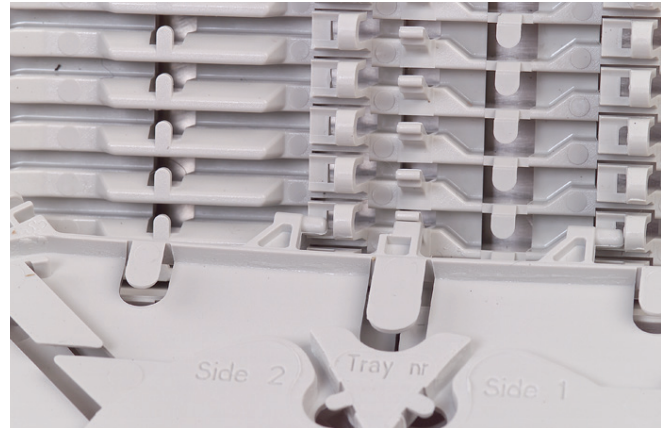
3.2 To remove push the two snapfits at S2 UMS-profile and slide the wraparound plate towards S1 UMS-profile.
