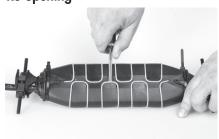
1 Cut off the tie wrap(s). Remove the springs.
