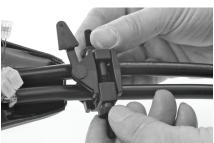
5 Install the gliders in the strain relief block(s). Mount the nuts and tighten them simultaneously (by hand).
