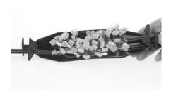
4 Position the non-pivoting strain relief arm(s) in the smaller half shell. Put the splice into the half shell and the cables in the strain relief block(s). Check if the splice is centered in the gel surface.
