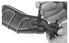
8 Install the top arm(s) of the strain relief block(s) on the bigger half shell. Install the tie wraps (1 tie wrap for size A, 2 for size B and C) at the end(s) of the closure as shown on the picture. Tighten, using a pair of pliers. Cut off the excess.
