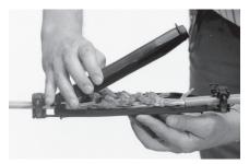
2 Remove the top arms of strain relief block(s). Gently open the closure.
