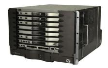
Managing the C4c CMTS is typically done via the SNMP or CLI interfaces. The C4c CMTS has multiple options available for IPDR, a useful tool for measuring bandwidth usage. Physical maintenance of the C4c CMTS is very simple. Air filters should be inspected and/or replaced per recommendations in the C4c CMTS User Guides.
