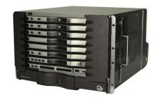
The C4c CMTS provides cable operators with significant improvements in DC power consumption per downstream channel as compared to other compact DOCSIS 3.0 platforms. This leads to reduced powering and cooling requirements for the operators' facilities, which can provide savings in operational and capital expenditures.
