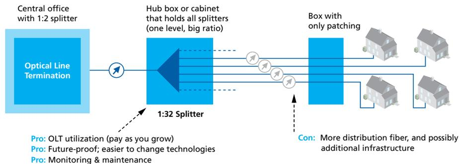
**Centralized:** A centralized split strategy uses a single layer of splitters, typically 1:32. These splitters are fed by the fibers exiting the optical line terminal (OLT) ports in the CO and distribute individual fibers to each premises. The splitter is typically connectorized and located in an outdoor cabinet or FDH or spliced into an OSP fiber-optic splice closure.
