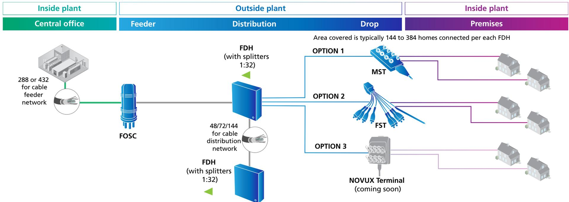
As the number of fibers in the distribution and access portions of the network increases, the ability to manage them in the CO is critical. The key tool for managing high-density fiber connections in the central office is the optical distribution frame (ODF). How your ODF is configured can make a big difference. The FTTH ePlanner will guide you in determining the best CO connectivity solution for your application.
