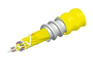
Fiber indoor cable, TeraSPEED® Plenum MPO Trunk, interlocking aluminum armored with plenum jacket, Singlemode G.652.D and G.657.A, 48 fiber multi-unit with 12 fiber subunits, Yellow jacket color, Feet cable marking
