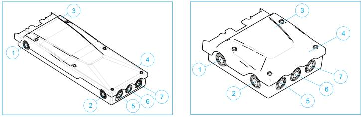
3.1 If a conduit fitting is required, drill hole along side or bottom using a hole saw bit. Reference pre-molded knock outs for conduit location and placement. Conduit can be installed to all sides except the top.
