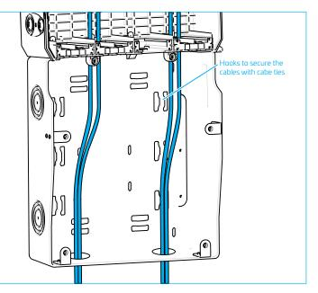
4.1 Arrange the cables and the pigtails in the SKIRT with respect to their bend radius
