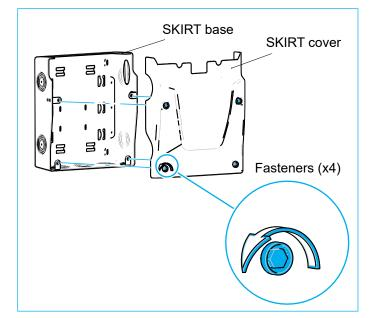
1.1 Rotate fasteners counterclockwise to unlock and lift off the cover.
