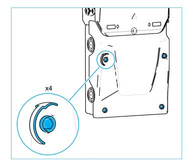
5.1 Re-mount the cover of the SKIRT and rotate the fasteners clockwise to lock. Refer to the BUDI-M installation instruction for cable and pigtail installation. Assemble BUDI-M cover to BUDI-M box.
