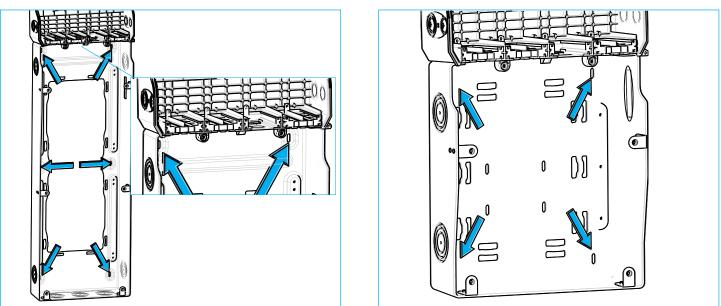
2.1 Place the SKIRT against the wall, with its top surface flush with the bottom of the BUDI-M box. **Note**: center the SKIRT with the BUDI. Leave at least one inch space between the bottom of the SKIRT and the final grade for cover removal. If a duct for dropcable is present, position it in the lower right quadrant of the skirt opening.
